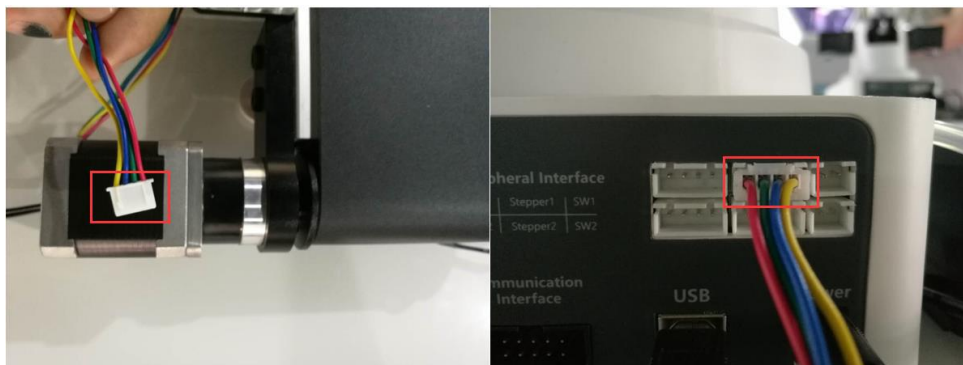
Figure 2.2 Conveyor Belt connection
